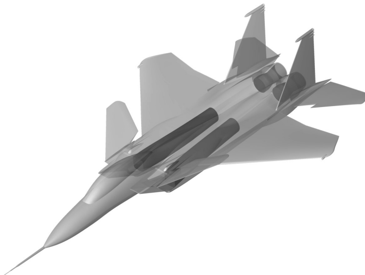
Figure 9. Modified F-15 with engine duct geometry.
