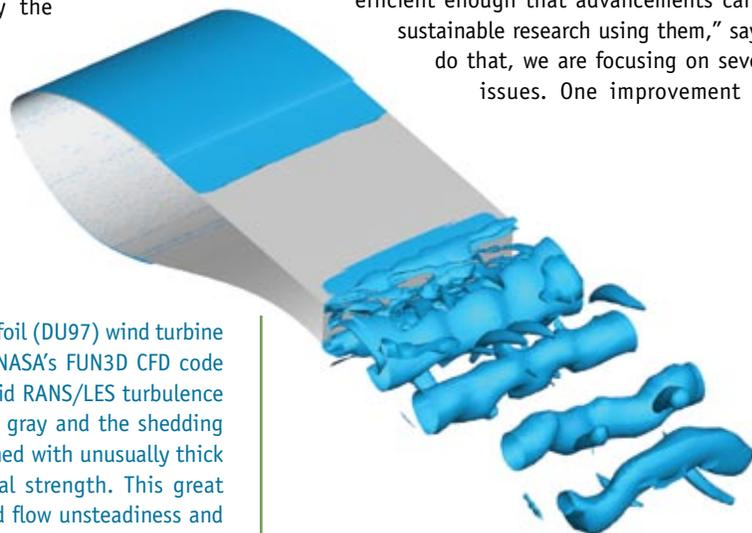
Simulation of an infinite-span "flatback" airfoil (DU97) wind turbine airfoil designed by Delft University using NASA's FUN3D CFD code modified by Georgia Tech to include a hybrid RANS/LES turbulence model. The airfoil geometry is shown in gray and the shedding vortices in blue. Flatback airfoils are designed with unusually thick bases intended to increase their structural strength. This great stiffness comes at the expense of increased flow unsteadiness and possible increased noise.
