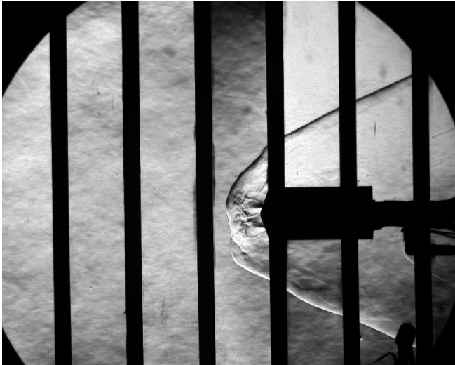
Figure 25 – Sample Schlieren image for the tri-nozzle configuration at M_\infty = 4.6 , \alpha = 0 -deg, and C_T = 1.0
