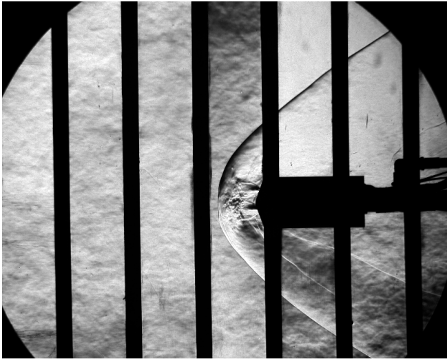
Figure 24 – Sample Schlieren image for the tri-nozzle configuration at M_\infty = 2.4 , \alpha = 0 -deg, and C_T = 1.0
