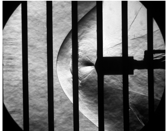
Figure 23 – Sample Schlieren image for the center nozzle configuration at M_\infty=2.4 , \alpha = 0 -deg, and C_T = 4.0
