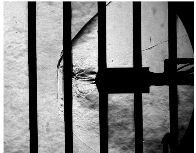
Figure 27 – Sample Schlieren image for the quad-nozzle configuration at M_\infty = 2.4 , \alpha = 0 -deg, and C_T = 3.0
