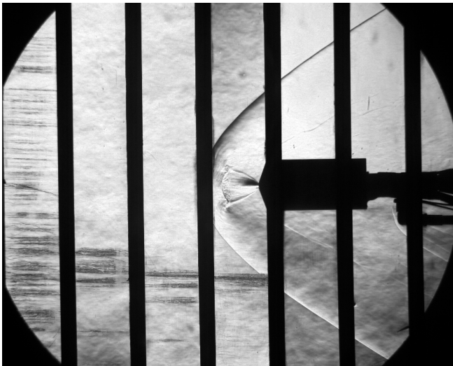
Figure 21 – Sample Schlieren image for the center nozzle configuration at M_\infty=2.4 , \alpha = 0 -deg, and C_T = 1.0
