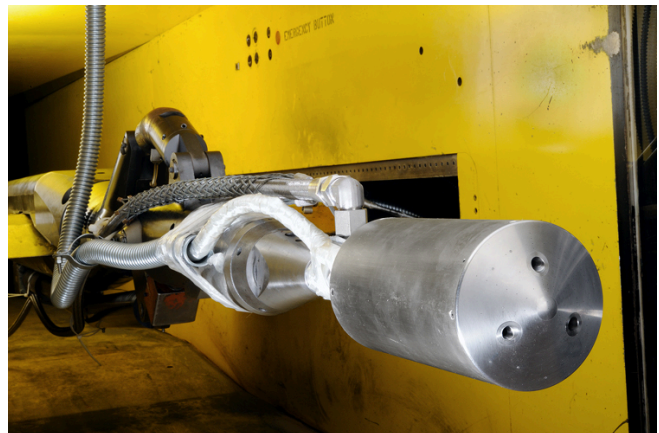
Figure 17 – Installation photo showing the tri-nozzle configuration with high-pressure & instrumentations lines
