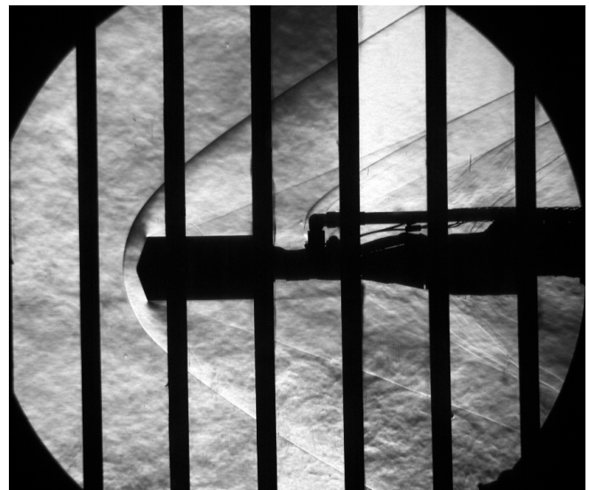
Figure 19 – Sample Schlieren image for the baseline configuration at M_\infty = 2.4 and \alpha = 0 -deg
