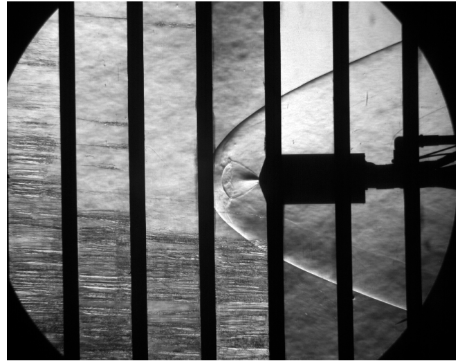
Figure 22 – Sample Schlieren image for the center nozzle configuration at M_\infty=4.6 , \alpha = 0 -deg, and C_T = 1.0
