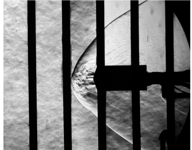
Figure 26 – Sample Schlieren image for the quad-nozzle configuration at M_\infty = 2.4 , \alpha = 0 -deg, and C_T = 1.0
