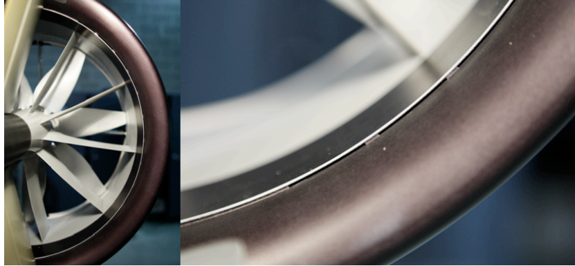
Figure 20: Coanda Trailing Edge Flow Control, with Close-up of Slot Geometry
