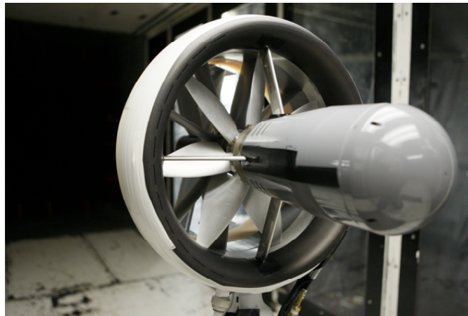
Figure 21: Leading Edge Flow Control Configuration in the Wind Tunnel
