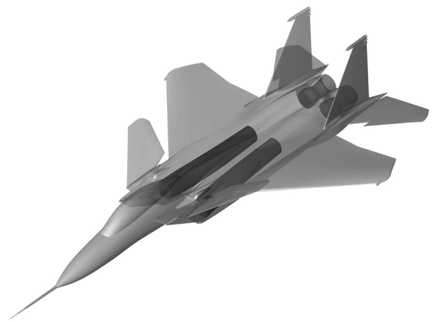
FIGURE 3. MODIFIED F-15 WITH ENGINE DUCT GEOMETRY. TAKEN FROM [38].
