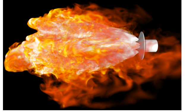
Fig. 8: Retropropulsion simulation performed on Summit. Freestream flow direction is from left to right.
