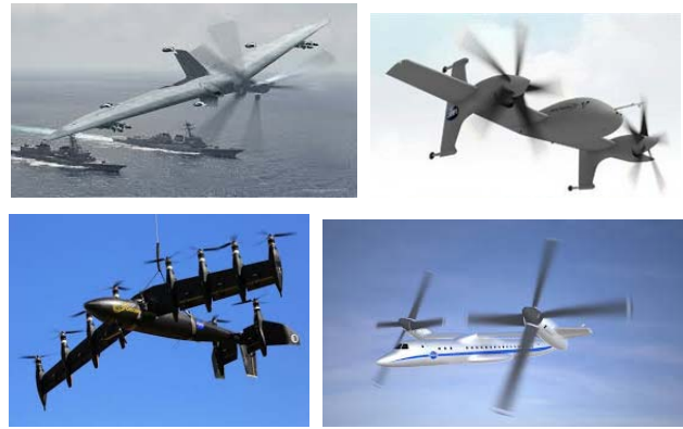
Figure 3: Advanced tailsitter or tilting rotor/wing concepts currently under study – upper left, Northrop Grumman TERN aircraft; upper right – Sikorsky blown wing tailsitter; lower left – NASA tiltwing UAV; below right - NASA Large Civil Tilt Rotor (LCTR) concept.
