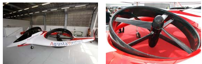
Figure 8: Agusta-Westland Concept Zero tilt duct demonstrator aircraft (left) and close-up of the Concept Zero tilting ducted rotor (right).
