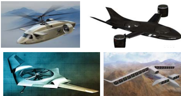
Figure 1: Advanced V/STOL vehicles with ducted rotors or fans currently under study – upper left, AVX Coaxial Compound Helicopter (propulsion); upper right - Boeing Phantom Swift (lift and propulsion); below left – a notional DARPA “flying wing” vehicle with lifting rotors embedded in the airframe; below right – an Aurora Flight Sciences high speed VTOL.
