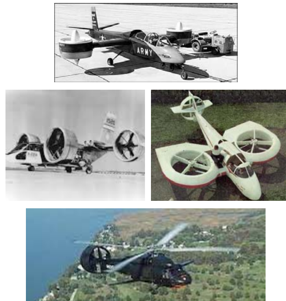
Figure 7: Four past lifting fan V/STOL systems – the Doak VZ-4 tilt-duct (left), the Bell X-22 tilt-duct (center left) and the Vanguard Omniplane (center right); and the Piasecki X-49 (below).
