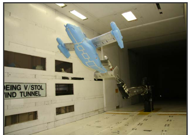
Figure 2. MV-22 BVWT 0468 high-angle-of-attack 0.15-scale wind tunnel model.
