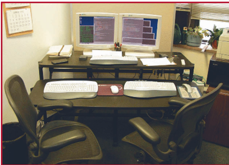
Figure 2. The pair programming station has two task chairs, a 60-inch-wide Anthro AdjustaCart, wireless keyboards and mice, and two LCD displays supporting a merged 2560 × 1024-pixel desktop. You can see the sustenance items—refrigerator, microwave, fresh-air supply, and plants—on the right.
