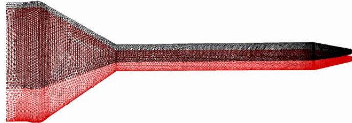
Red: Undeformed Surface Black: 1st Deflected Surface from FEM
